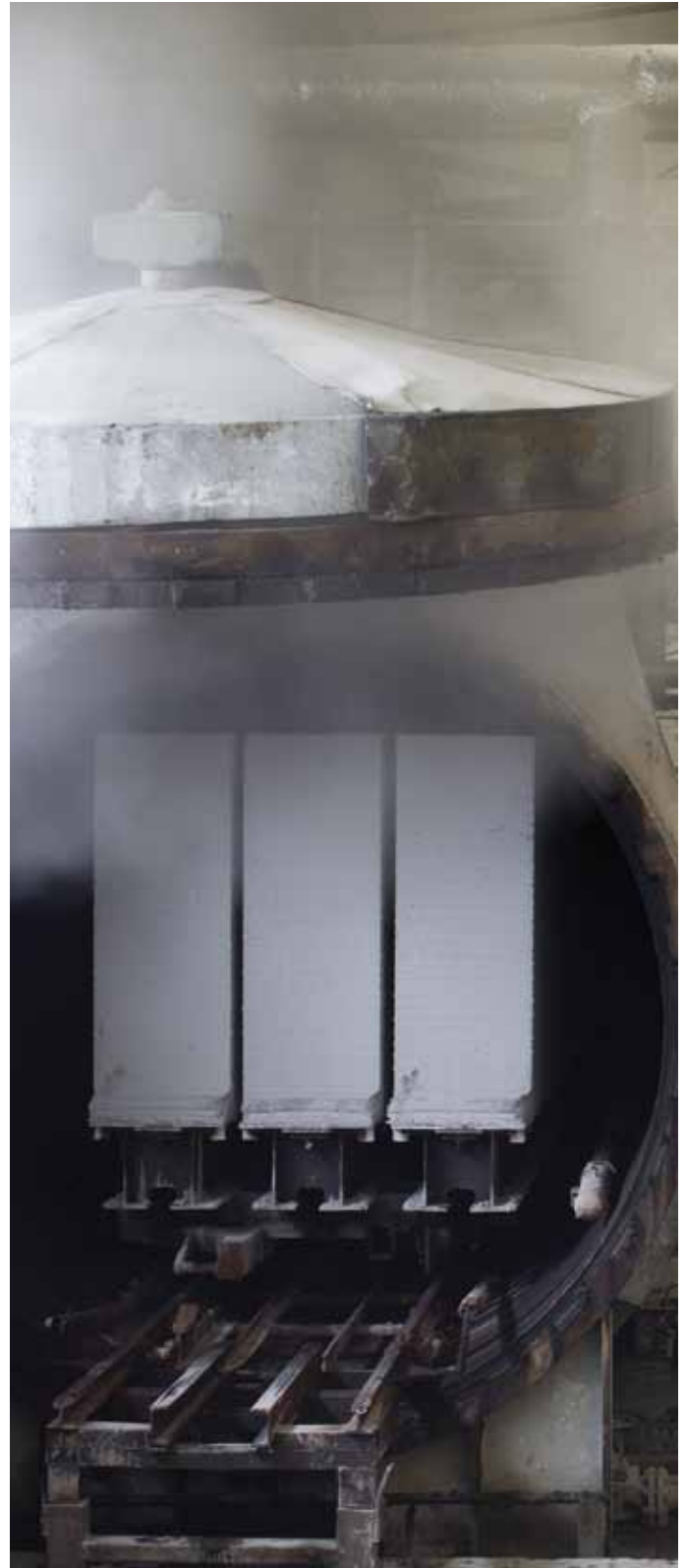
QUINN- lite Cakes ready to be removed from Autoclave.
