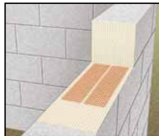
A layer of thin joint with reinforced mesh shown.
